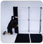
Slowly run your hands down the sides of the panel, attaching magnetic strips to the channel bars and straightening as you go.
