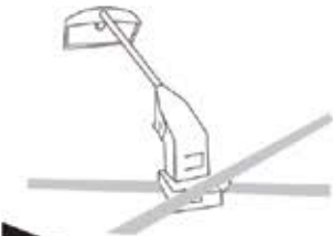
5 OPTIONAL Attach lights to top of frame by sliding the plastic "x blocks" under the frames cross sections.
